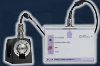
By connecting the EA014 Torque Measurement adapter to a Transmille calibrator, torque calibration capabilities can be added to your laboratory in a cost-effective manner.
