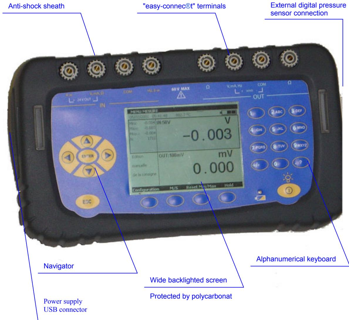
Calys 75 is delivered in standard with a strap and a stand for desktop use, a quick battery charger, and a set of 6 measuring cables with crocodile clips
