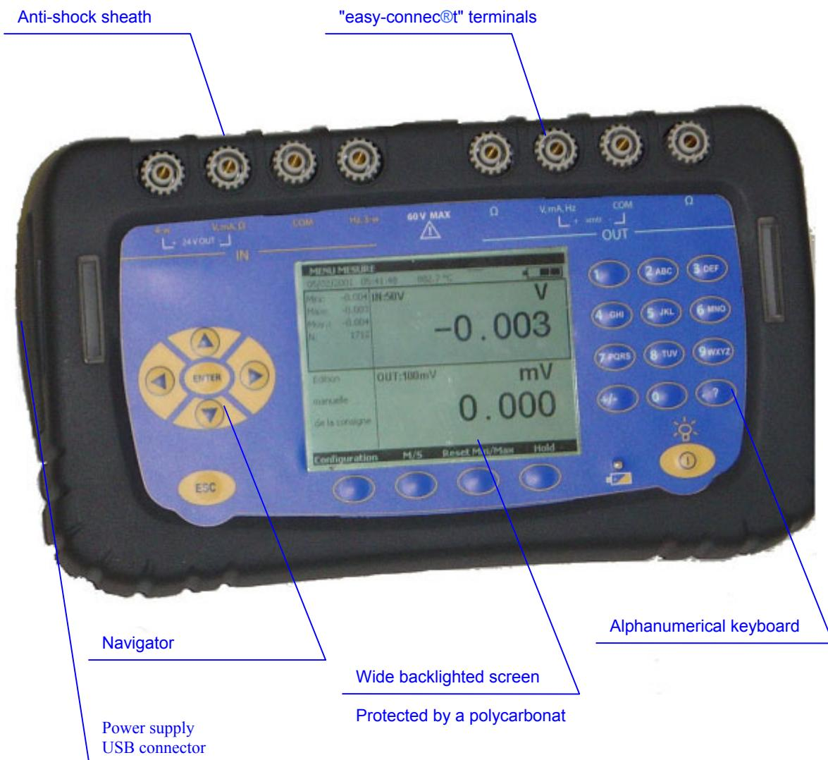
Calys 50 is delivered in standard with a strap and a stand for desktop use, a quick battery charger, and a set of 6 measuring cables with crocodile clips
